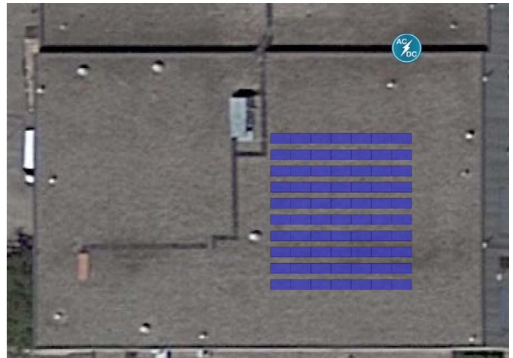
25kW Solar System on the Upper Roof of the Facility
