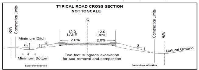
The preceding sketch is to be used as a typical cross section through embankment and excavation sections for all normal road construction. Wherever side roads and branch roads lead off of the main road, such roads shall have the crown of the branch road meeting the shoulder elevation of the main road. Side slopes shall retain a 1:3 or a 1:4 slope depending on the functional classification of the road.
