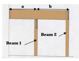
Use "a" to determine joist size and "a" + "2b" to determine beam and footing sizes. The length of "b" is restricted by both the length of "a" and the size of the joists.
