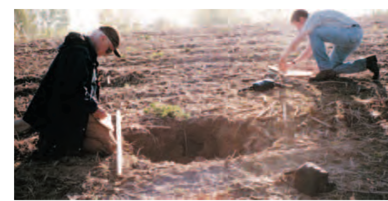
FIGURE 4. Sinkhole MN25-D0291, D291 was a 6-foot-diameter by 5-foot-deep vertical-sided collapse that formed after harvest in October 1996 in Welch Township. Field cultivation filled D291 in spring 1997 and 1998. It redeveloped each following autumn. Photograph contributed by Dan Bauer.
