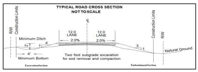
The preceding sketch is to be used as a typical cross section through embankment and excavation sections for all normal road construction. Wherever side roads and branch roads lead off of the main road, such roads shall have the crown of the branch road meeting the shoulder elevation of the main road. Side slopes shall retain a 1:3 or a 1:4 slope depending on the functional classification of the road.
