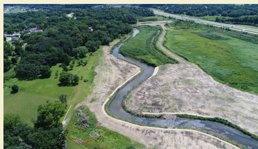
Streambank restoration projects reduce nutrient and sediment loading from the landscape and improve habitat.
